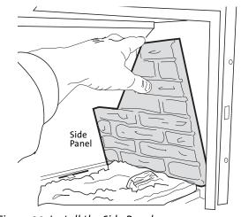
Figure 20. Install the Side Panel.
